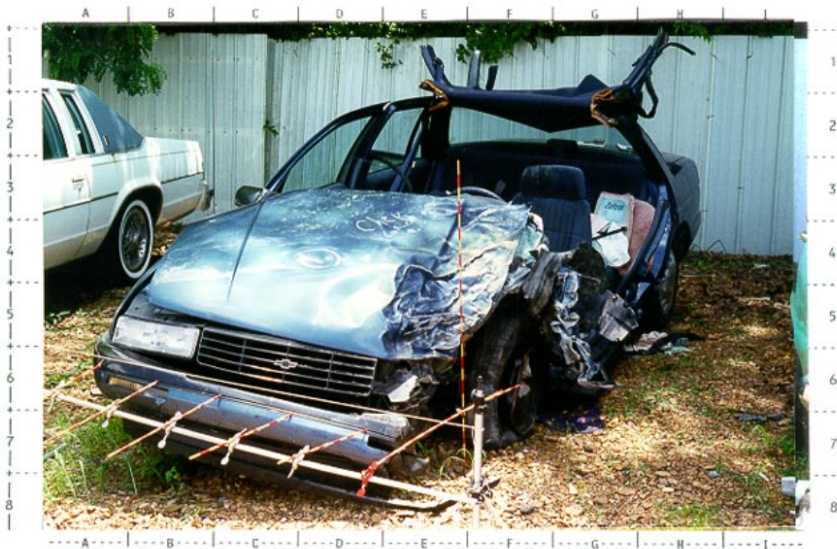
# 31 -- Front left view of 1991 Corsica's front left damage with contour gauge present; NOTE: peeled-back roof and cut L A- & B-pillars
